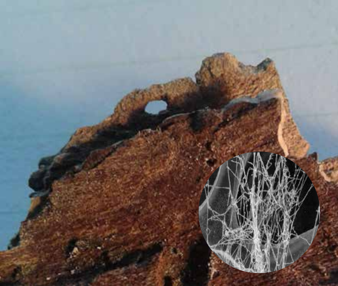
White Rot fungus on decaying North Shore pine log, common in damp locations everywhere.
